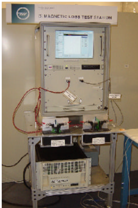
Figure: 2 A view of the loss testing system and the test fixtures
